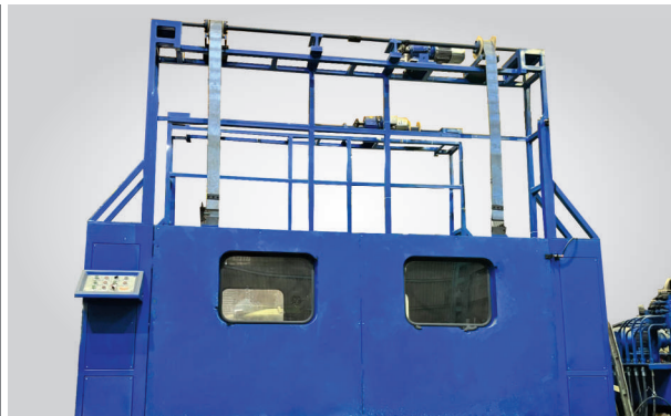
WHEEL CLEANING STATION
